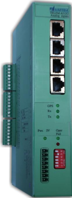
The TELEM family RTU module TELEM-AI12 with 12 analog differential analog inputs is used for measure 12 analogue values. Module bases on 16-bit DSP. It can be used as an independent RTU or in connection with other devices. Interfaces to other equipment are RS-232, RS-422 or RS-485. Data exchange protocol IEC 60870-5-1-101. Time synchronization with GPS receiver.
